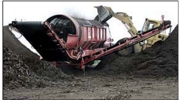
EDUARDO CONTRERAS / Union-Tribune A front loader was used to fill a screener with composting material at El Corazon Composting in Oceanside last week. The screener separates the material into grades of compost that will be sold to the public. The company has seen demand for compost grow.
